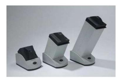
The Comparator System 2000 is based on a versatile 2-field visual comparator with an optional lighting unit to guarantee correct lighting conditions for colour grading and colorimetric analysis.
