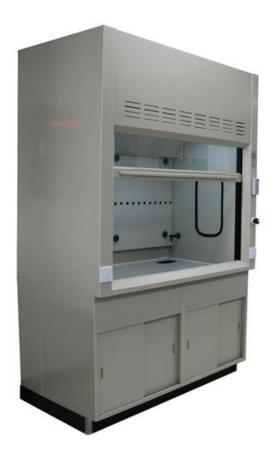
Featuring a particular assembling metal frame that can be easily dismantled. Front and rear uprights are made of aluminium draw pieces, chromium treated and painted with epoxy resins, acid and solvent resistant. Front upright shape is designed at a 45Ű angle section, for preventing any reversal airflow and the generation of air whirls.
