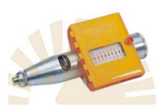
Measuring range 10 to 70 N/mmÂ<sup>2</sup> compressive strength. Impact energy = 2,207 Nm. Rebound values are recorded as a bar chart on a paper strip. One roll of paper strip offers space for 4000 test impacts. A bridge concreted in several stages is tested for uniform concrete quality. The engineer will perform a series of tests in intervals of 10 m each.
