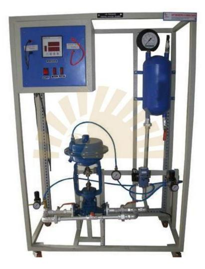
The Level Control System Trainer is the system which outlines the basics of closed loop level control process and other aspects related to it.
