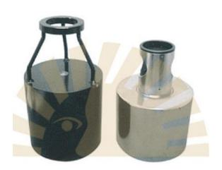
Each test hammer should be checked after 1000 test impacts. A testing anvil is used to check whether there bound test mechanism is working correctly. In case of values beyond the tolerance (due to contamination by very fine cement, wear or defects) cleaning or inspection will be required.
