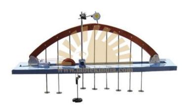
Experimental and analytical study of 3 hinged arch and influence line for horizontal thrust.
