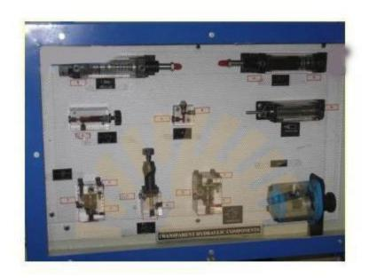
The setup consists of transparent body (or cut section) of the Hydraulic components which gives idea regarding the internal constructional features of the Hydraulic components. Following components are included in the trainer: Pressure relief valve Single Acting Cylinder(spring return) Double Acting cylinder Pilot operated pressure relief valve Telescopic cylinder. Pressure reducing valve Flow control valve Cut section of Gear pump Sequence valve.
