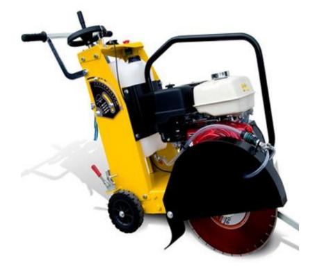
Driven by electrical motor or by engine as per customers requirement. Diamond bit of 100 mm to 600 mm maximum can be supplied as per requirement. The trolley in which the engine is fitted is supplied with cooling arrangements with the help of a water tank. Arrangements to control the depth is also provided. A safety guard is also provided on the diamond blade. Two wheels are provided for easy movability of the machine.
