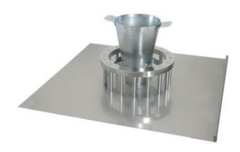
The J-ring test can be used to determine the passing ability of self-consolidating concrete. It is applicable for laboratory use in testing different concrete mixtures for passing ability or can be used in the field as a quality control test.
