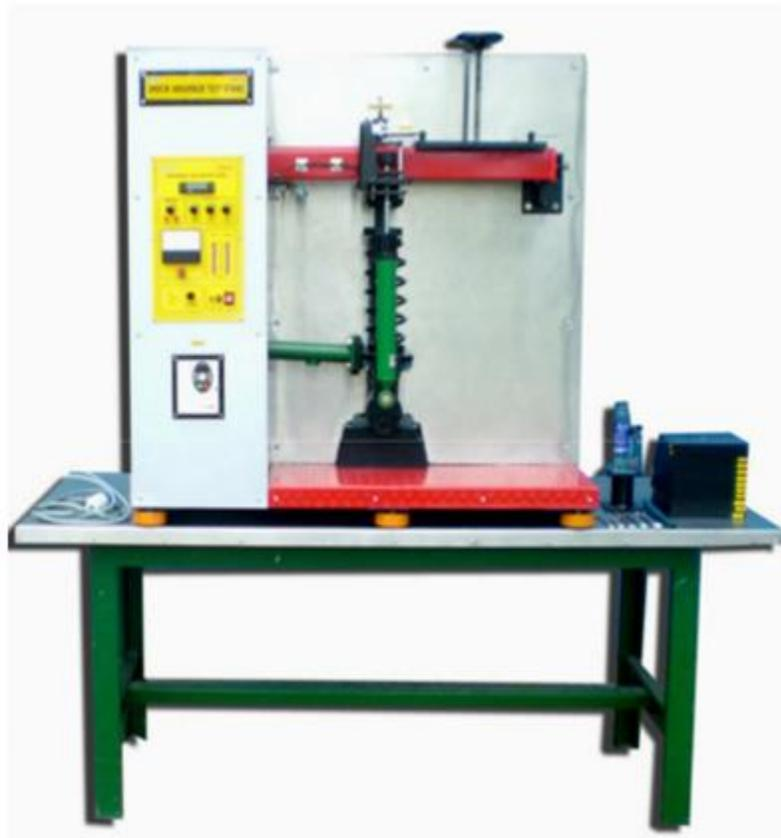
A trainer for suspension and shock absorbers featuring a computer for data acquisition of test data and analysis of results. The trainer explores the construction and performance of shock absorbers as well as the operation and characteristics of suspensions.
