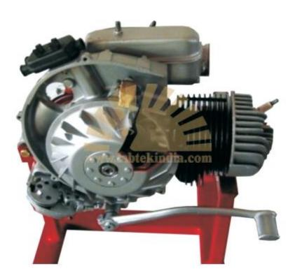
This model is made out of used BAJAJ engine, suitably sectioned to show the internal construction of the engine, gear box, clutch and rear wheel mechanism and the model is fitted on a sturdy iron frame. The complete internal details can be demonstrated by operating the kicker lever to show the working of the piston, sparks from the spark plugs can also be shown
