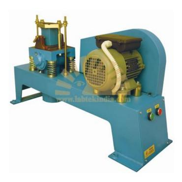
Vibrating Machine is used for vibrating the mix in moulds at a frequency of 12,000 ± 400 cycles per minute. The vibrator is mounted over 4 coiled springs and the vibrations are developed by means of a revolving eccentric shaft. The centre of gravity of the vibrator, including the cube mould, is either at the centre of eccentric shaft or within 25mm below it. The simple design of the machine facilitates easy assembly and dismantling of the cube moulds.
