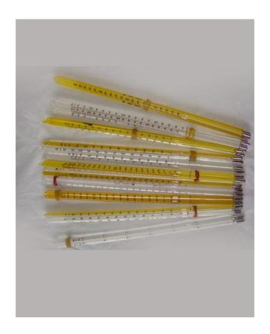
Chemical thermometers made up of high class glass capillary with prominent mercury or alcohol column as per requirement for accurate results for Research Laboratories, Institutes, Schools, Colleges, General laboratories in private sectors. Range available between -100° C to +600° C consumer should indicate the specified range, least count, accuracy class. We can also supply according to the customer drawings & samples.
