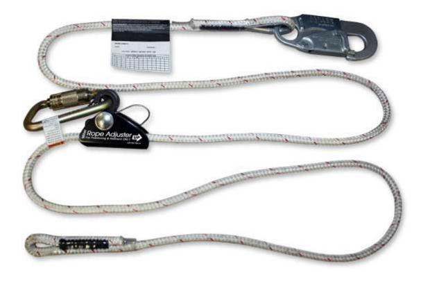
Linking the user to protection and bridging the missing gaps. 'ZI' offers a wide variety of polyamide rope and webbing lanyards to be used as a connecting element or component of a arrest system. All link connecting rope lanyards are made up to 12mm dia, 3 strand polyamide rope. The splices are protected with a sleeve. The length of lanyard is always measured from one load bearing point to other load bearing point in an unloaded but taut condition.
