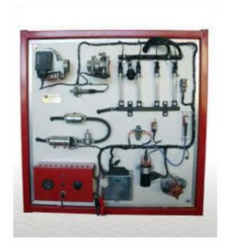
The Four-Cylinder Engine trainer should consist of a complete, fully operational Multi Point EFI system. Original components should be utilized and clearly laid out on a display board that is mounted on an integrated floor stand, made from powder coated electro galvanized steel, mounted onto wheels for mobility. A color coded schematic chart, under a lexon polycarbonate protective screen, of the EFI system and circuit's, should also be mounted onto the trainer for reference.
