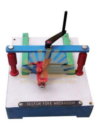
The experimental unit is used to generate and investigate pure harmonic reciprocating motion.
