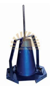
The slump cone in these slump test apparatus is filled with freshly mixed concrete and tamped with a tamping rod in three or four layers. The top of the concrete is leveled off with the top of the slump cone, the cone is lifted vertically up and the slump of the sample is immediately measured.
